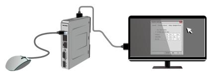
When mTV is powered up and displays image, click the system setting button. (Default System Password: 111111) It is necessary to connect the mTV to your network through a RJ-45 cable.
